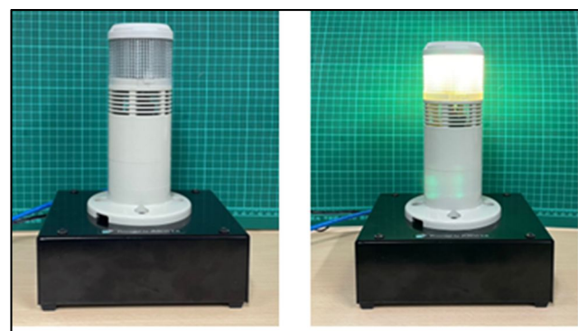
Fig. 10. Documentation of warning light triggered by demo EEW.
