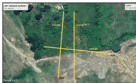
Fig. 3. Design of the SRT survey lines drawn in a satellite image of the area taken in 2022.
