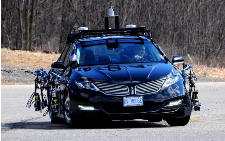
Fig. 1. Measurement System at the Waterloo Test Track: M. Van Gennip, Vehicle Dynamic Modelling and Parameter Identification for an Autonomous Vehicle. Master of Applied Science, University of Waterloo, December 2018 [9].
