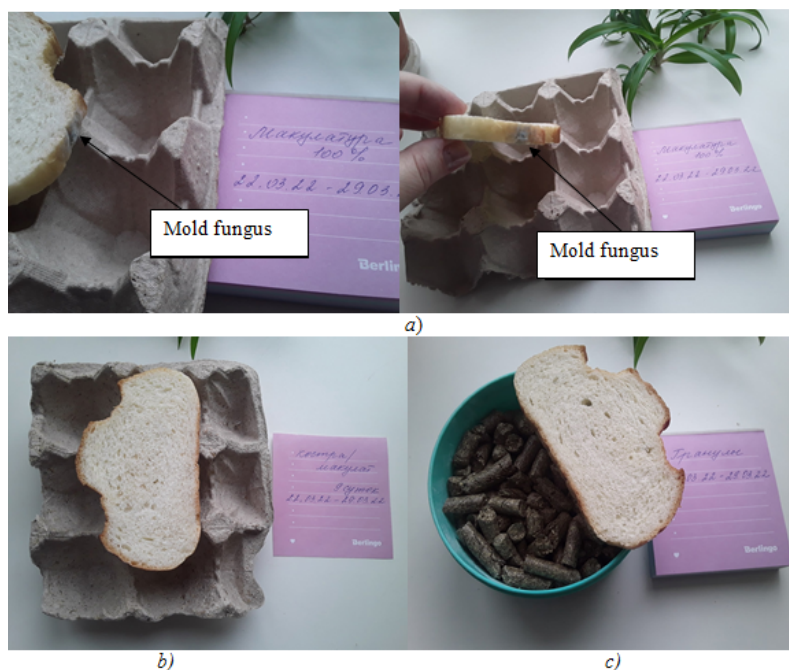
Fig. 9. The development of mold fungi on a loaf of "Podmoskovny", stored on substrates of different composition: a) on a lumpy egg pad made of 100% waste paper; b) - on a lumpy egg pad made of 50% waste paper and 50% flax shives; c) - on pallets of shives flax flour M – 560 ("Compiled by the authors").
