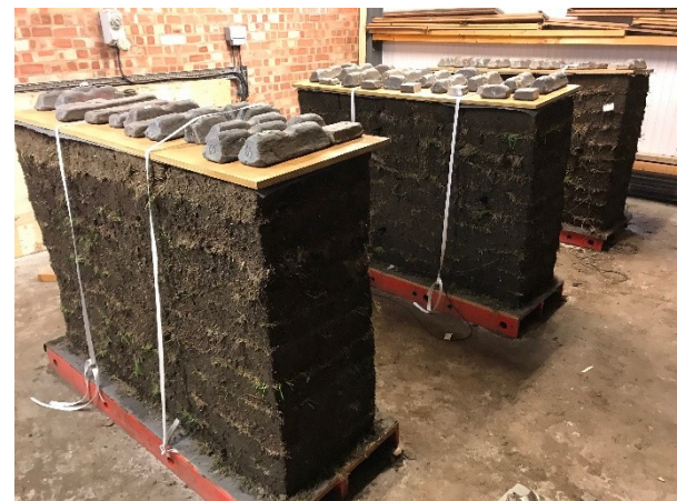
Fig. 1. Turf walls manufactured for compression testing (under a 2 kPa surcharge)
