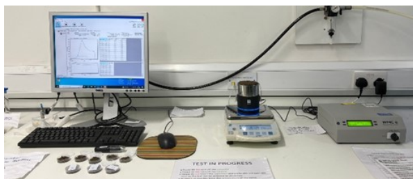
Fig. 2. Control PC (left), HYPROP (middle), WP4C (right).
