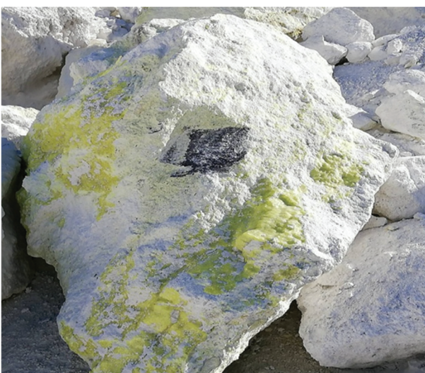
Fig. 5. Sulphur crystalline aggregates hosted in a white silica sandy deposit, used as silica additive in the clinker production of cement. Kastriani quarry of Heracles cement company (LAVA SA).
