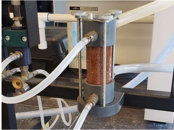
Fig. 7. Constant head permeability test
