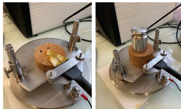
Fig. 2. Preparation steps for the Hot Disk measurement.
