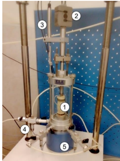
Fig. 6. Sample placed in the stabilometer test chamber: 1 - sample in a sealed chamber filled with water; 2 - S-shaped dynamometer; 3 - displacement sensor; 4 - water pressure sensor in a sealed chamber; 5 - retractable piston.
