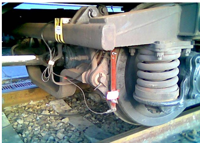
Fig. 5. The Installation of measuring equipment on the car.
