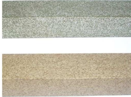
Fig. 5. Protective and decorative coating obtained by microplasma electrolytic oxidation.
