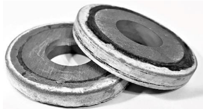
Fig. 3. Abrasive wheels with a cutting layer of mineral-ceramic material.
