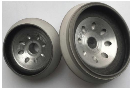
Fig. 1. Friction unit of a spinning machine modified by microplasma oxidation.
