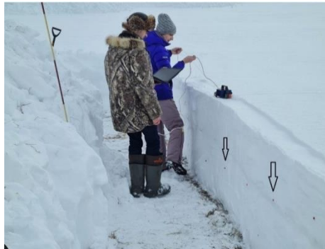
Fig. 4. GPR survey of snow cover using metal reflectors (markers) (indicated by black arrows), 25.02.2022.
