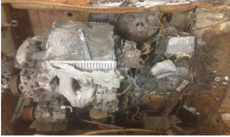
Fig. 1. General view of the burnt engine compartment.
