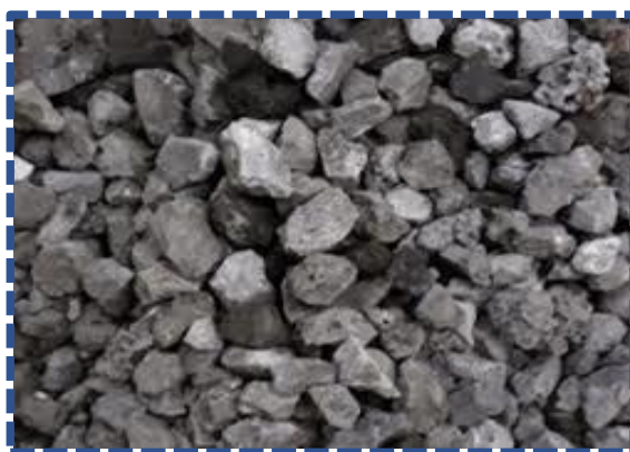
Figure 3: A typical example of a furnace slag
