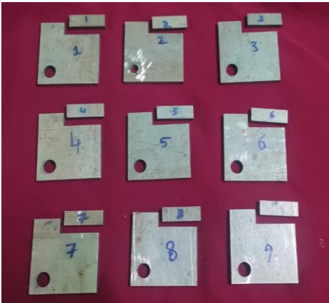
Fig.2. Specimens after cutting with Wire EDM
