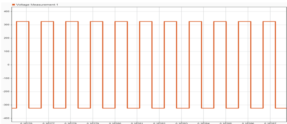
Fig 4 Output voltage waveform of open loop inverter
