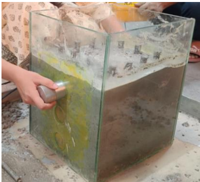
Fig. 5. UPV measurements at 3 sections
