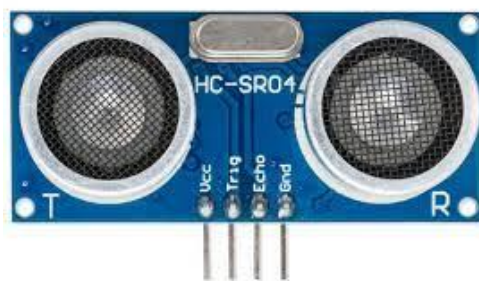
Fig. 1. Ultrasonic sensor (hc-sr04 module)
