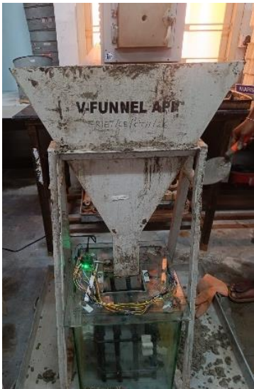
Fig. 3. Test performance while filling the glass column
