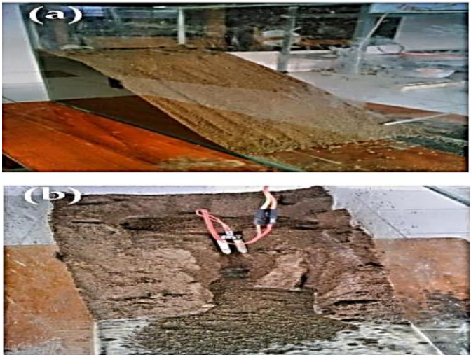
Fig. 5. Landslide simulation before (a) and after (b) the event in soil with sensors
