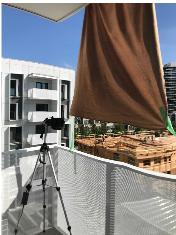
Figure 2: Photo of camera setup during the experiment. To minimize movements between photos, the camera was mounted on a tripod and shielded from the direct sunlight to prevent overheating. The operator manually pressed the camera trigger for each photo.
