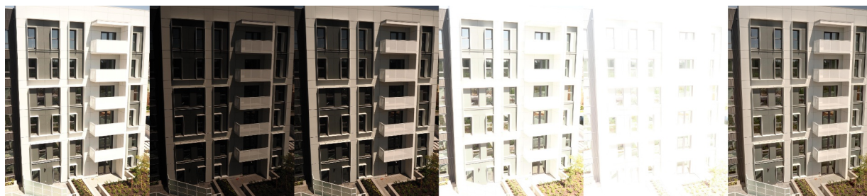
Figure 3: Five bracketed images and reconstructed HDR image (right). The left image shows the original exposure, followed by four increasing exposure times. The reconstructed image shows much better tonal information in shadows and washout regions compared to the original bracketed images.
