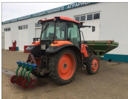
Fig. 2. Multifunctional unit (MFA) for harrowing crops with simultaneous fertilizing
