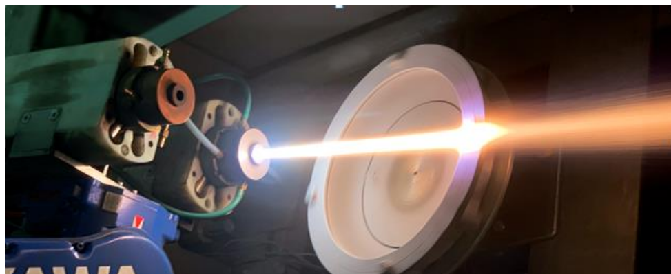
Fig. 1. Supersonic air-plasma spraying of a wear-resistant coating WC/10Co4Cr on the working surface of a hydraulic equipment part.
