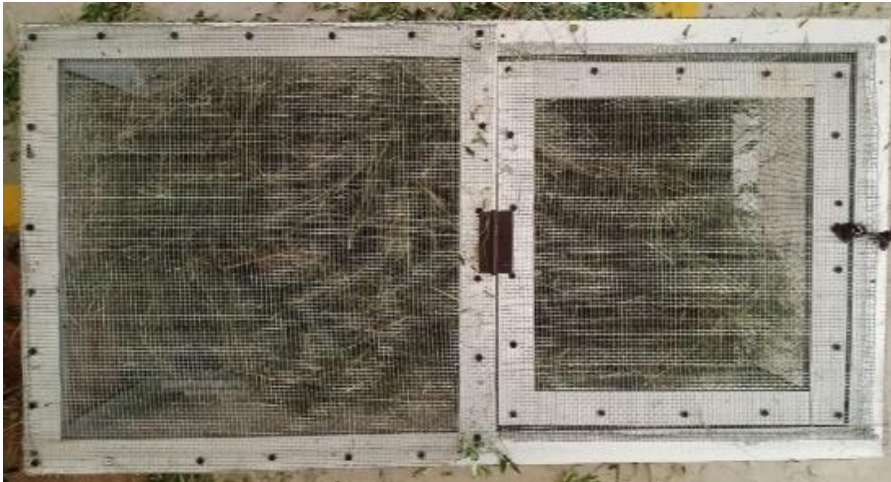
Fig. 2. Bed drying chamber
