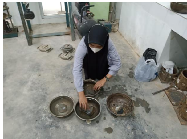
Fig. 2. One of the stages in the specific gravity and water absorption test of coarse aggregate
