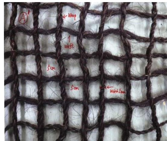
Fig. 2. Examples of dunula nets (fiber) with mesh dimensions of 5cm x 5cm, and 5mm thick.
