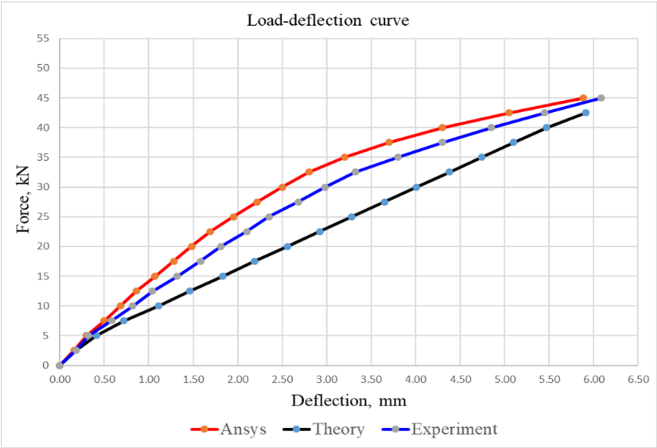
Fig. 10. Load-deflection curve for Series 1
