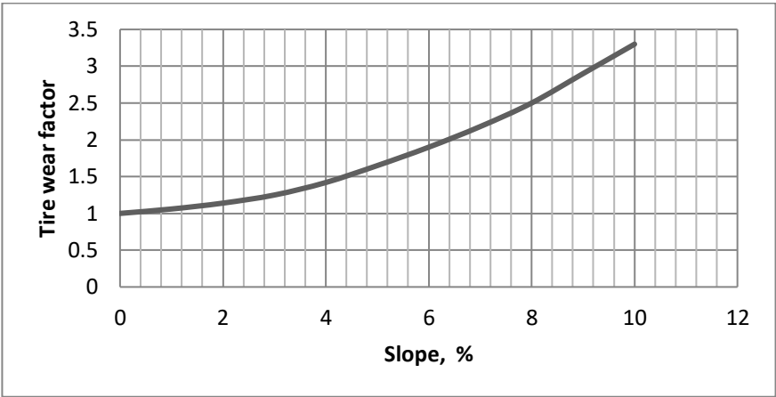
Fig.2. Dependence of the relative wear of tires on the value of the longitudinal slope
