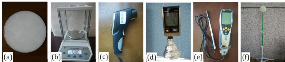
Fig. 2. Experimental instruments or devices: a) Naphthalene test specimen, b) electronic balance, c) infrared thermometer, d) temperature and humidity recorder, e) hot-wire anemometer, f) homemade bracket according to Yaping Cui, Jingchao Xie, Jiaping Liu, Peng Xue. [5]
