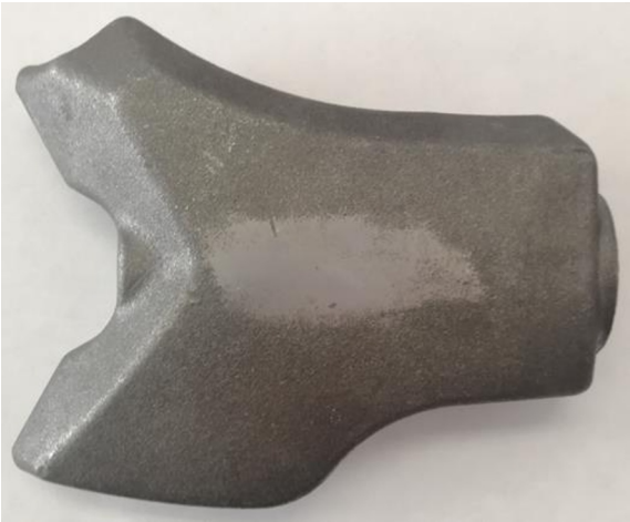
Fig. 2. Left side cutter with scraper.
