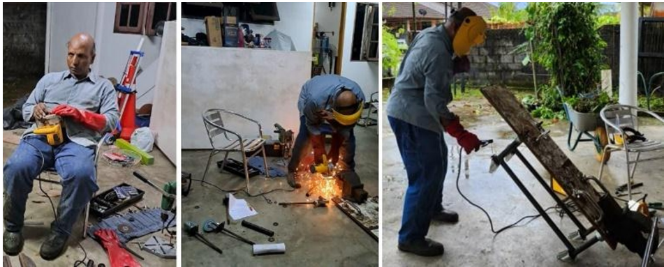
Fig. 8. Rebuilding the work bench with more steel members onto the workbench to increase the strength of it.
