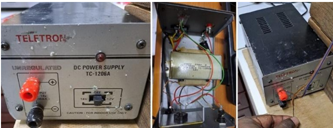
Fig. 11. The power supply for the DC motor which can supply 12V or 14V; the blade turns faster and with more power at 14V.
