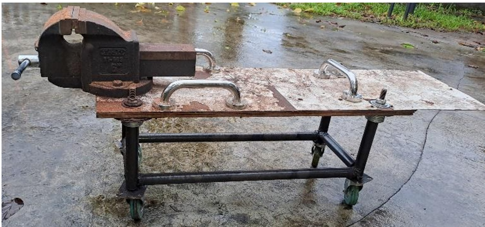
Fig. 9. The workbench with wheels, handles and sufficient steel members welded to make it very sturdy to move over uneven earth near a tree or plant. The vice must be retracted to move it else there the center of gravity will shift inappropriately.
