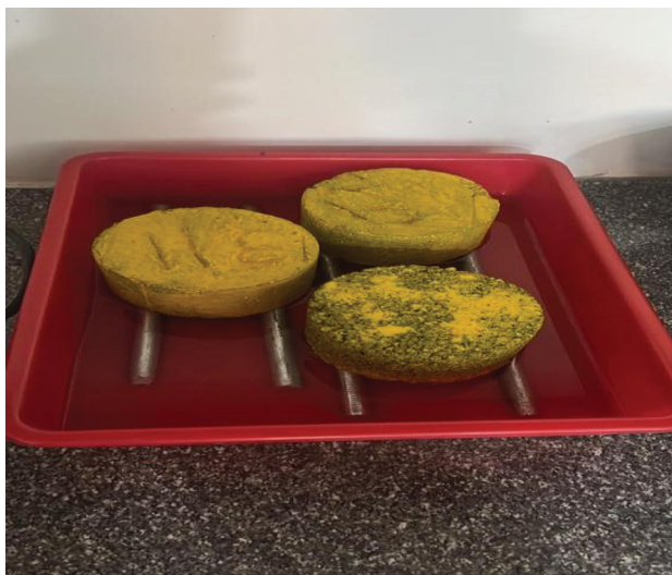
Fig. 3. Specimens used for the acid attack test
