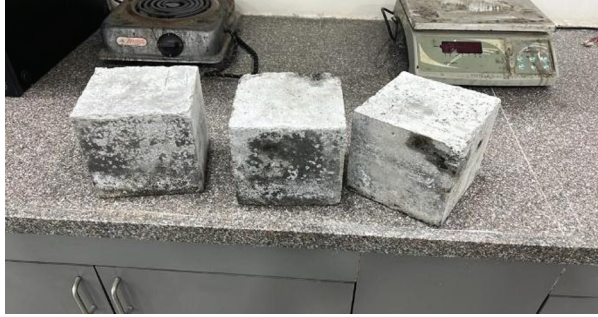
Fig. 2. specimens used for the sulphate attack test
