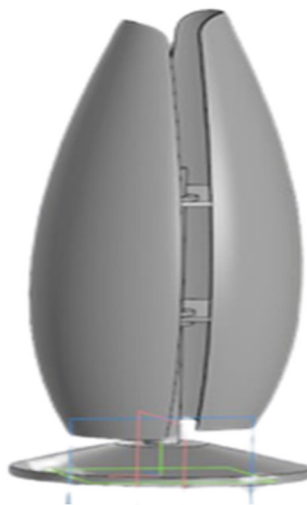
Fig. 2. Scheme of the Savonius-Orthogonal wind generator.
