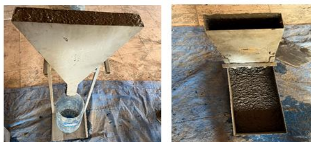
Figure 2: V-funnel and L-box experiments of study mixtures.
