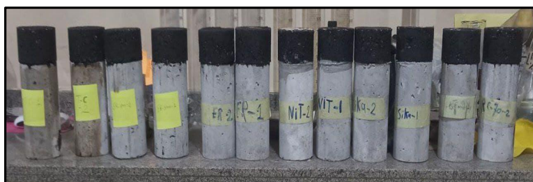
Figure 1: Composite Specimens used in a direct shear test.
