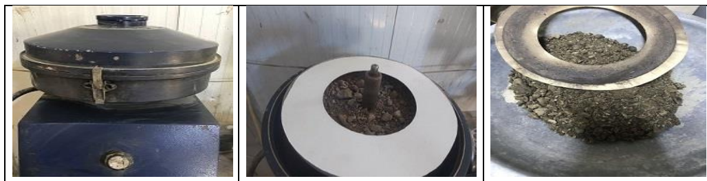
Figure 2: Centrifuge Extraction test: (A) Extraction machine, (B) before and (C) after testing.
