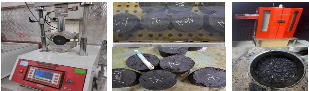
Figure 7: Marshall Sample preparation and testing.
