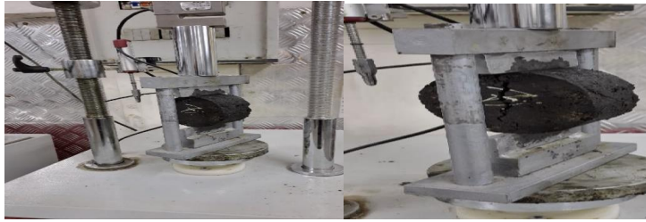
Figure 8: Indirect Tensile test of neat and nano-modified asphalt mixture.
