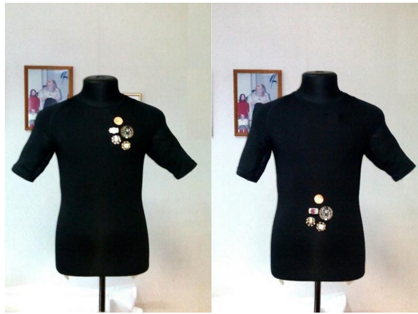
Fig. 8. Prototypes of a tight-fitting rashguard with embedded PCB
