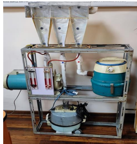
Fig. 2. a)-technological scheme. 1-Air drive pump, 2-Rashodomer, 3-Colorifer, 4-Thermometer, 5-Experiment device, 6-Psychrometer, 7- U-shaped manometer. b) actual view of the experimental device.
