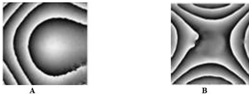
Fig. 6. Interferograms of deformations during the heating of a white plastic plate obtained at different times after the start of heating: A - interferogram of deformations of the plate made of white plastic, heating time 1 min; B - interferogram of deformations after 4 min of heating.
