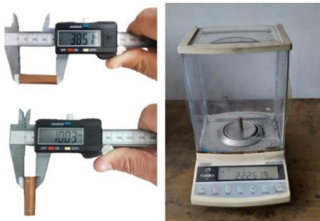
Fig. 3. Dimensions and weight of the developed EDM tool (Courtesy: NITTTTR, Chandigarh)
