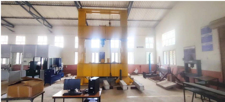
Fig. 5. Beam placed for loading frame of 100 Ton capacity
