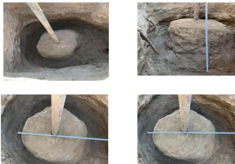
Fig. 13. Photo of measuring the geometric dimensions of the fortified subsidence soil.
