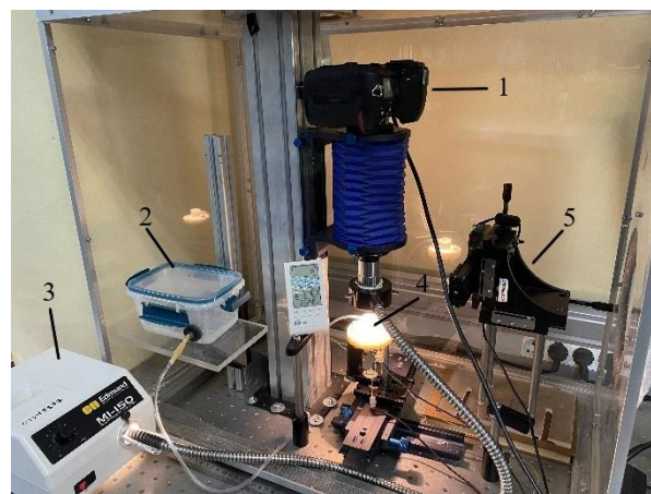
Fig. 3. The photo of the experimental setup: 1 – digital camera, 2 – container with working liquid, 3 – light source, 4 – test section, 5 – confocal sensor.
