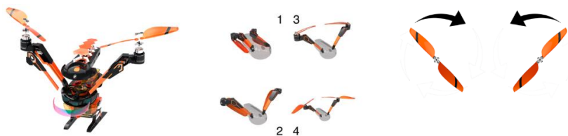
Fig. 5. Diagram showing the phases of opening the drone's wings.
