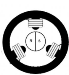
Fig. 6. The structure of the brushed motor.
