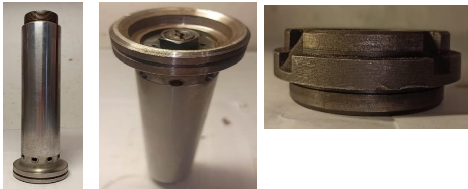
Fig. 2. The wear of the axle box of the hydraulic vibration damper, the piston rod and its guide
