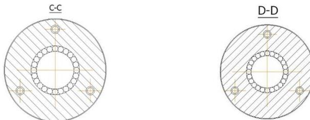
**Fig. 8.** C-C and D-D views of the construction of the device for stretching non-ferrous metal wires into a cylindrical shape with the help of balls
