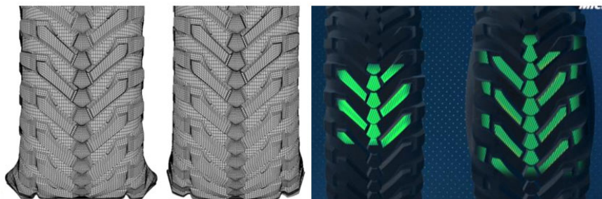
Fig. 10. Michelin Ultraflex tyres at low and normal pressures.
