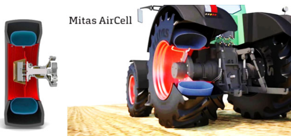
Fig. 9. Mitas Aircell tyre principle of operation.
