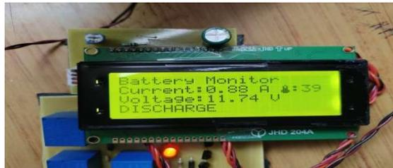
**Fig. 7** DISCHARGE OF BATTERY ON THE LCD DISPLAY WITH VOLTAGE READING AND TEMPERATURE DISPLAY
