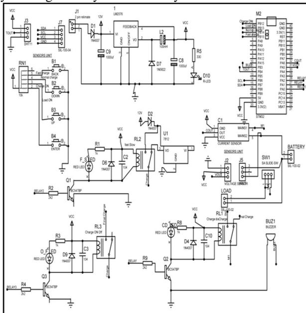
**Fig.3.** Circuit Diagram of BatteryManagement System
