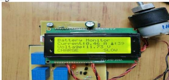
**Fig.5** DISPLAY OF BATTERY WHILE SLOW CHARGING
