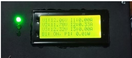
Fig.7. LCD display when the battery is used.
