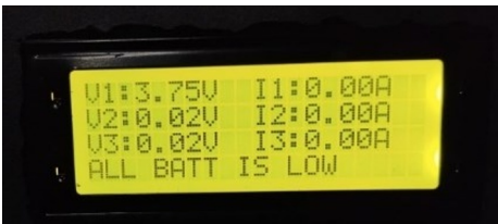
Fig. 8. LCD display when all batteries are off.
