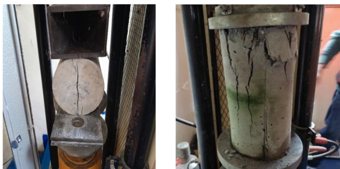
Fig. 2. Testing of compressive strength and tensile strength of concrete
