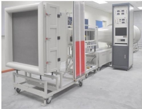
Fig. 3. Longwin LW-9300R Subsonic Wind Tunnel located at The National Defence University NDUM [29].
